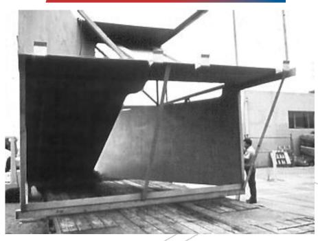
Komax large-scale channel mixers are designed to be installed in water treatment channels of any cross-section including open and closed ducts. Low pressure drop design can be provided in complete assemblies or in component form where access is difficult.
